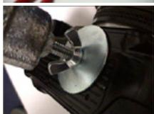
Use your fingers to tighten the wing nut on the mounting. DO NOT use a wrench. You may risk stripping the threads on your camera or breaking the tripod mount. Both are equally bad.
