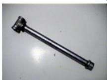
This first step is pretty easy. Just attach the tee and end cap to one of the pipes to form a basic handle. Feel free to tighten these parts together as much as you like. I recommend using the vise and a wrench. Don't use your hands, you'll just hurt yourself and not get it tight enough.
