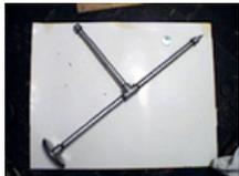
Lastly, take the remaining two pipes, screw them into the T joint of the handle, and attached the base and the mounting. And your done! You can tighten these parts as much as you'd like. Either give them a good hand tightening or the full fledged vise and wrench tightening. The only reason not to do the vise-wrench tighten is if you want to be able to collapse this or swap components. You can vary the pipe lengths and barbell weight however you like.
