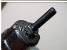
You'll want to make this really tight because this is where your camera attaches. You want it tight not because it'll fall off or anything, but because putting the camera on and taking it off requires lots of turning action. If it loosens, the bolt will pivot around as will your camera making hard it to keep still. If this happens while you're filming, you'll have to stop and find a wrench. This [schematic view](#) may be a little clearer than the pictures.
