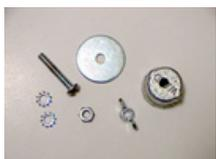
The mounting requires the parts in the picture on the left. Bolt, two lock washers, flange washer, nut, wing nut, and a drilled end cap. Put a lock washer on the bolt and the put it through the end cap with the bottom of the bolt coming out of the top of the outside of the end cap like in the middle picture. Put another lock washer on and then the nut. Put the end cap in the vise and tighten with a wrench. The lock washer will keep the bolt from turning.
