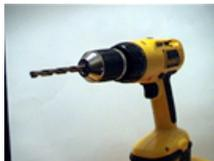
You'll need drill and a 1/4" drill bit that can go into galvanized steel. So, cheap wood bits will probably not survive this project. This happens to be a very nice drill in this picture, but any power drill will do.
